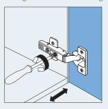
**3.** To adjust the fronts to make them closer to the cabinet, tighten or loosen the hinge screw at the back.
