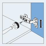
**2.** To move the fronts slightly to the left or right, tighten or loosen the hinge screw at the front.
